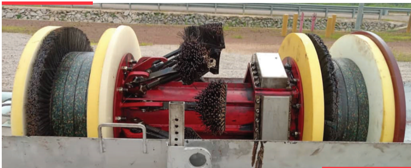
Cleaning pig – High performance wax bulldozer
